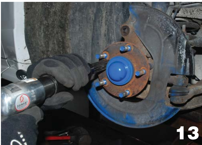
The tool's design allows it to fit around a stud and get into the recess area where the stud passes through the hub face.
