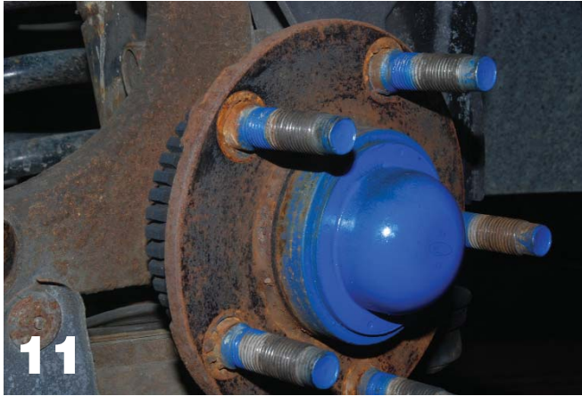
Look at the corrosion buildup around the studs. This must be cleaned up before installation of the new performance rotors. Failure to do so will surely cause a problem in the near future.
