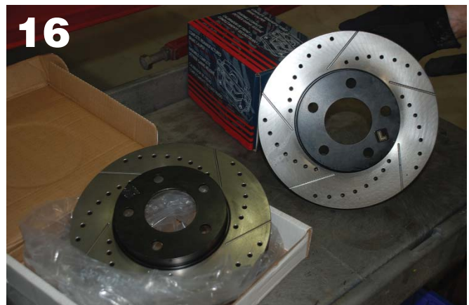
Here is a performance drilled and slotted rotor for the Mustang. There are differences in drilled and slotted rotors. Where the slots are, their angle and the location of the holes make a difference in cooling and removal of brake dust during operation. In addition, the quality of the metal is key to overall quality.
