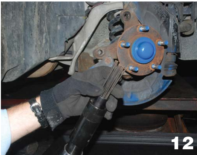
This de-scaling tool should be a "must-have" for every shop. It is one of the best ways of removing rust and scale buildup and works extremely well on hubs/studs and around the center raised area.
