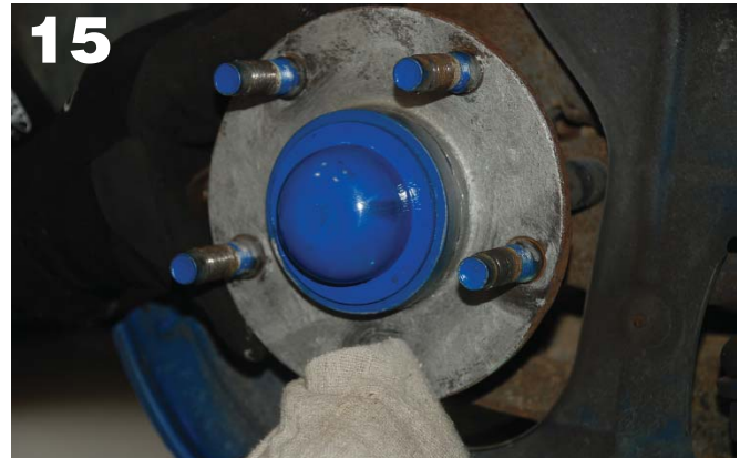
Many technicians believe in coating the hub face with a product such as the anti-seize compound used here to prevent rust and scale buildup. What you use is open to discussion, but I believe you should use something to prevent future buildup.
