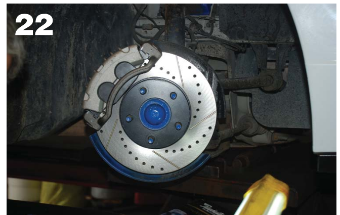
Here is the front brake, consisting of a new drilled and slotted performance rotor, a caliper with performance pads, a new mounting bracket and new hardware. This brake is a performance upgrade.
