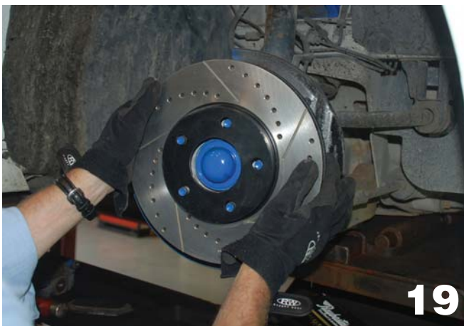
The technician slips the cleaned rotor onto the hub.
