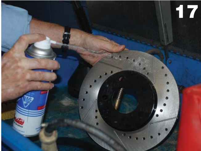
Depending on the protective coating used, you may need to clean a new rotor with an aerosol brake cleaner before installation.
