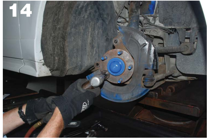
After the de-scaling tool is used, the final cleanup of the hub face is done with a tool such as this one. This tool also works well but doesn't remove heavy rust and scale as a de-scaling tool does. Likewise, a de-scaling tool doesn't leave as smooth a surface as this tool does. Doing the job correctly requires both tools.
